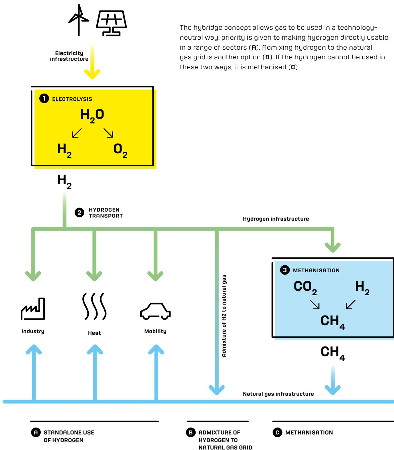
The hybridge concept allows gas to be used in a technology-neutral way: priority is given to making hydrogen directly usable in a range of sectors (A). Admixing hydrogen to the natural gas grid is another option (B). If the hydrogen cannot be used in these two ways, it is methanised (C).
